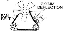
Figure 13. Fan Belt Tension
